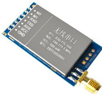
E50-TTL-500 is a 500mW wireless transceiver module(UART),with transparent transmission mode, operates at 148-173.5MHz(default 170MHz),TTL level, WOA(Ultra low power consumption) , strong ability of diffraction and penetration, suitable for complex environment.
